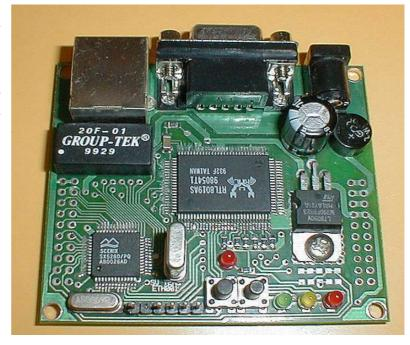
Three another LEDs HL12...HL10 connected to the Ethernet chip and mean "Collision", "Rx", "Tx" (from left to right).
