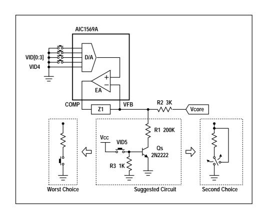
In the above figure, "Suggested Circuit" is a little complicated but much more reliable than the "Second Choice". R2 is the original resistor used with Z1 to accomplish the compensation network. Adding an R1 resistor effectively divides the feedback voltage. This also causes the compensator to increase the output voltage. VID5, Grounding of R1 depends on the control circuit
